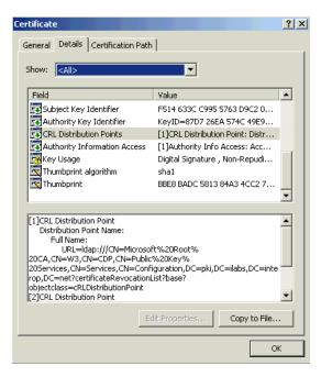
The starting point for the CRL is the CRL Distribution Point (the CDP), which is a field located in each certificate. The CDP is optional, but most well-run PKI installations include a CDP in each certificate. In the screen shot to the left, you can see the CDP we put in our iLabs demonstration certificates issued by the Microsoft Windows 2000 CA. In this case, the CRL has two distribution points, one available using an LDAP server and the other stored on an http server.
