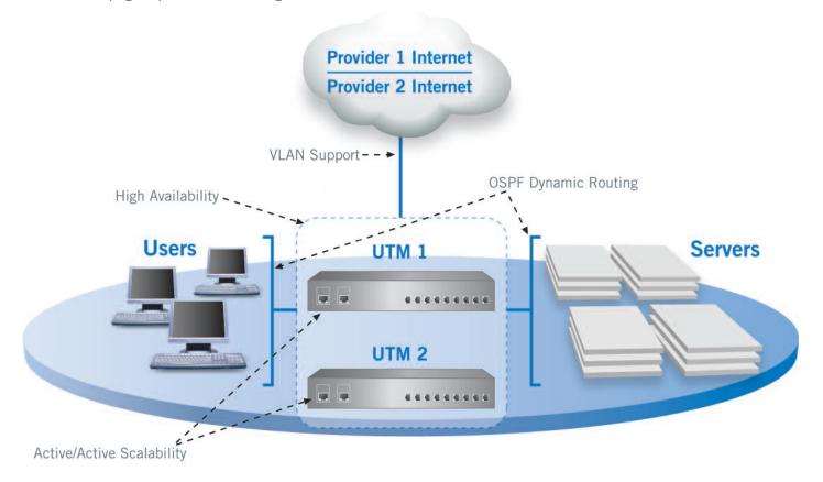
Enterprise-class UTM must smoothly integrate into the existing network, which means that features such as dynamic routing and VLAN support are required. Well-designed scalability and high availability strategies are also needed to support the needs of enterprise networks.
