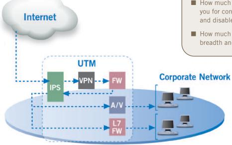
Flexibility in UTMs gives the network architect the option to have security services where they make sense, not in a fixed order. For example, an IPS might see traffic twice: once before it's decrypted to mitigate DoS attacks, and then again after it's passed through the VPN and firewall to look for different types of threats.
