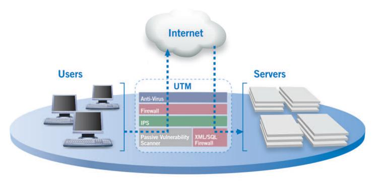
UTM supports consolidation by integrating multiple security functions into a single device. A critical requirement of a consolidated device is the capability to direct traffic flows through the UTM device, activating different functions, because not every security function applies to all flows.
